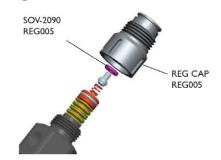
Then ease the cap down over the bobbin assembly ensuring the O ring Reg 060 enters the bore without damage or nicking. Once fully over the bobbin some green high strength thread locking compound can be applied to the thread and the cap screwed down. The cap can then be tightened down with a "C" spanner (Gedore No.40), the grub screw Reg 070 is then screwed in using a 1/16th allen key.
