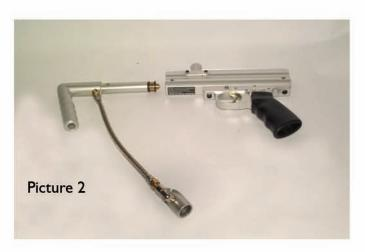
Stage 2 Remove valve body assembly (part No.1305) As shown in picture 2
